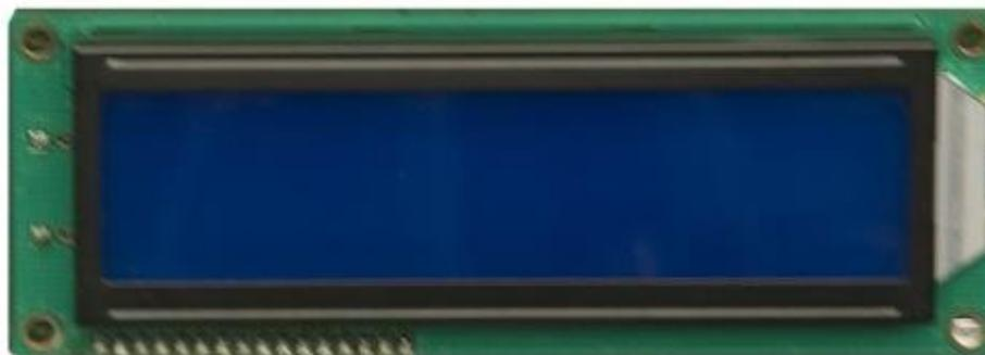
Display Lcd 2x16 SDEC P-S2E16VCT
